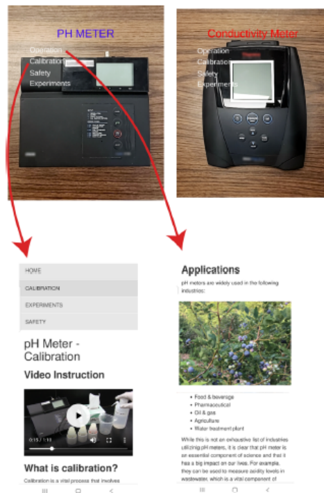
Figure 2.1. Screenshots of instrument recognition by the ARiEL application on an Android phone and the resulting connections to example, mobile-optimized web pages.
